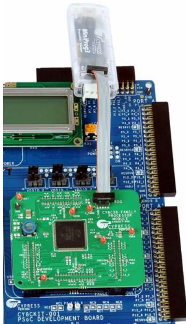
Figure 2-14. Connect MiniProg3 to J5 on the CY8C38 Family Processor Module
