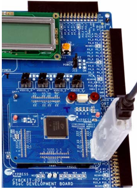
Figure 2-8. Connect MiniProg3 to J5 on the CY8C29 Family Processor Module
