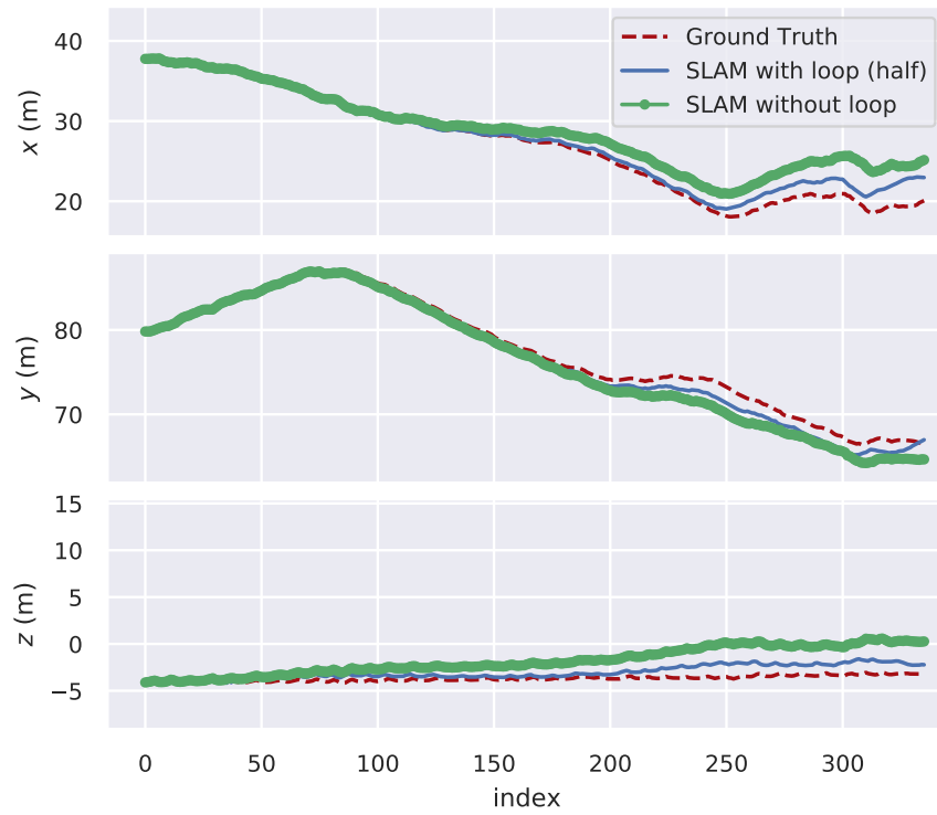
Figure 4.11: Comparison of trajectories with and without loop closure using RTAB-MAP with Kinect v1. The trajectory is plotted in meters for each axis (the z axis is aligned to gravity), against the camera frame index.
