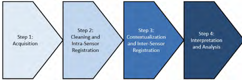
Figure 2.1: Generic workflow for utilizing 3D data capture techniques for remote environment observation.
