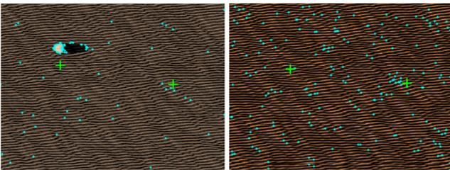
**Fig. 6** Placement of centroids on simulated sonar images. Features are displayed as cyan points, and the two centroids are the green plus symbols. Features associated with an object (left) will on average be closer to a centroid than features not associated with an object (right)
