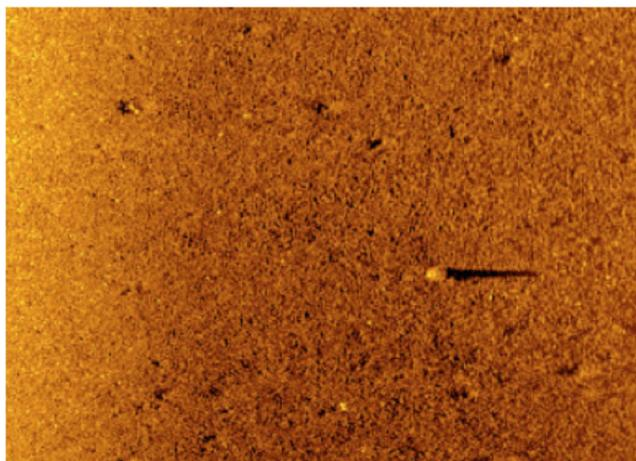
Fig. 2 SAS image of the seafloor with an object appearing prominently in the centre right
