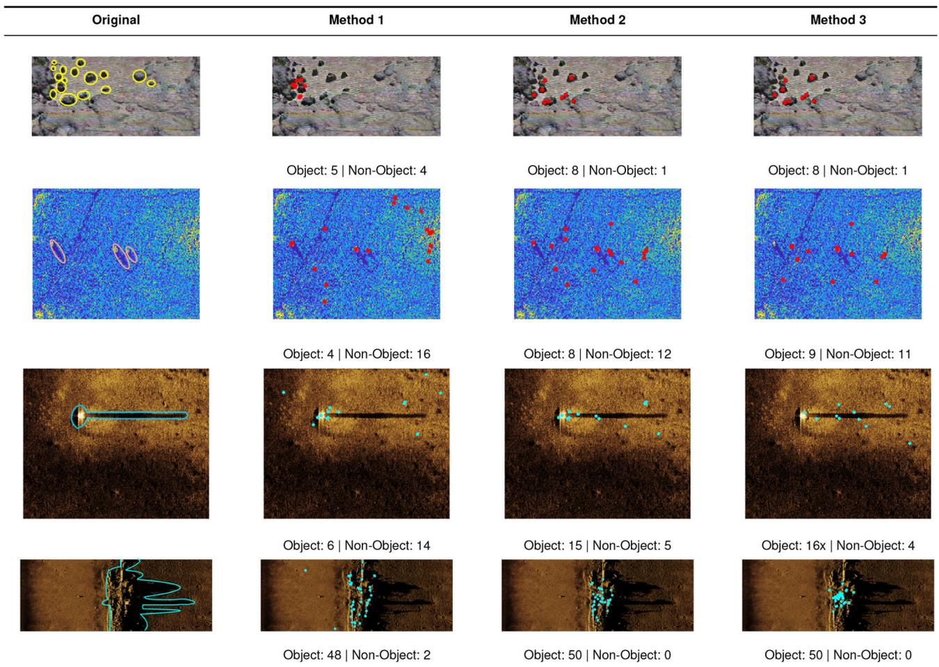
Fig. 10 Target detection methods on real sonar images with the SURF detector
