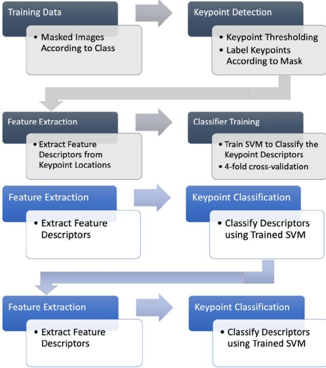
**Fig. 4** Feature classification. The first flow chart represents training an SVM model, and the second flow chart represents performing classification using that model
