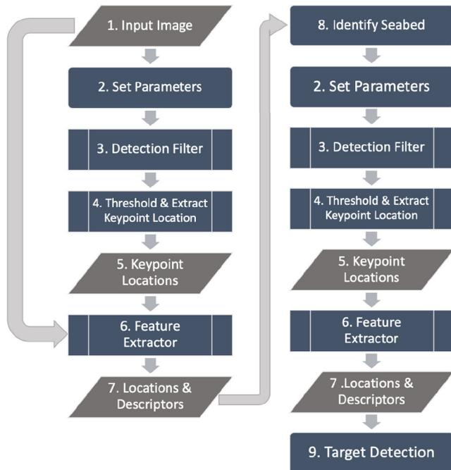
Fig. 3 General framework for our feature-based detection algorithm
