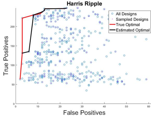
**Fig. 8** Example of a design space exploration. The red line shows the true set of optimal designs, and the black line shows what was estimated utilising only the magenta points
