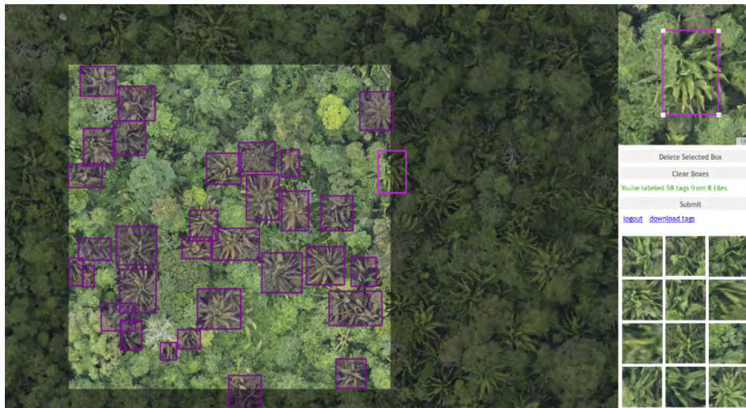
FIGURE 4.2: Labeling tool in action. Note that you are shown surrounding area of the tile allowing the user to label palm trees that overlap two segments. Thumbnails on the lower right allow easy visual grepping of currently labeled trees
