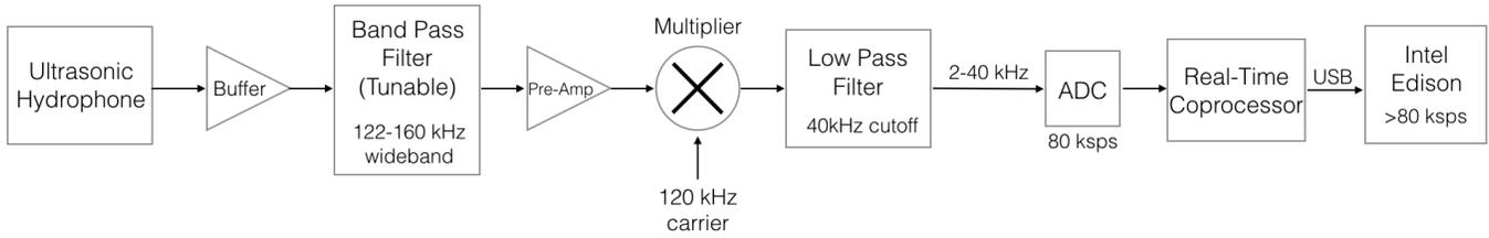
Fig. 7. Analog Filtering Circuitry
