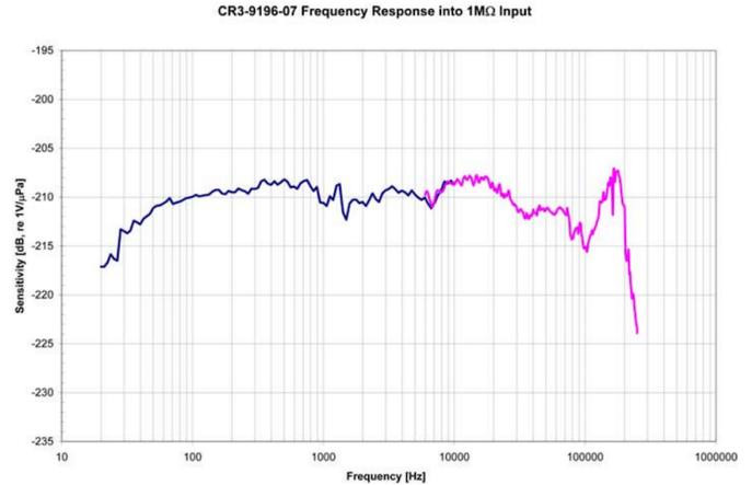
Fig. 5. Frequency response of CR3 Hydrophone from Cetacean Research Technologies, taken from[16]
