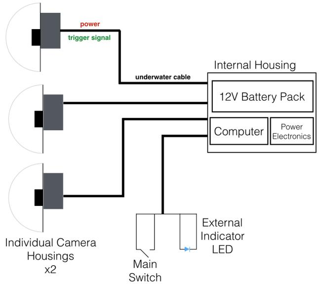
Fig. 4. Modular mechanical design of camera system, with each component housed in a separate enclosure
