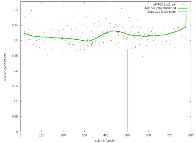
Fig. 9. MTF values across the columns of the image plane, with just the lens and without dome
