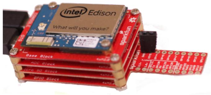
Fig. 3. Intel Edison Platform, with breakout boards for console, GPIO, microSD, and ADC (custom boards not pictured)
