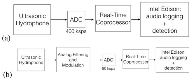
Fig. 6. Two configurations of acoustic recording and triggering system. (a) is used to record and process the entire 20 Hz to 200 kHz band of acoustic data at the Nyquist rate of the signal, removing the step of modulation. (b) is used to process only the desired frequency band and modulate the signal to a lower frequency for reduced power consumption.
