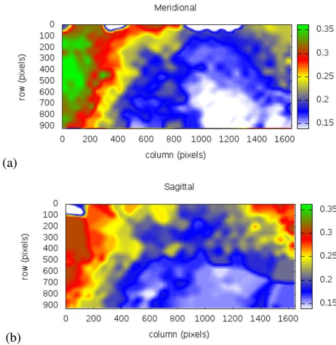
Fig. 10. 2D representation of MTF values for camera dome and lens system
