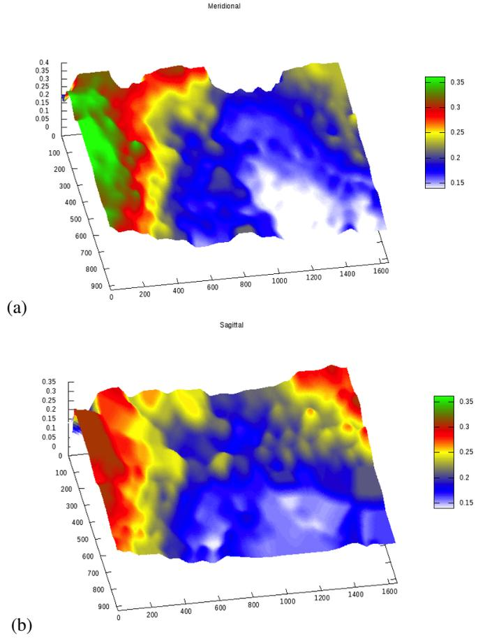
Fig. 11. 3D representation of MTF values for camera dome and lens system
