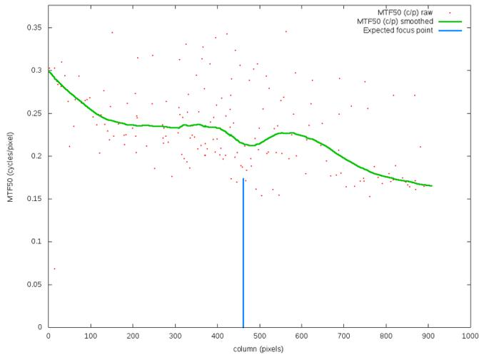
Fig. 8. MTF values across the columns of the image plane, with complete lens and dome setup
