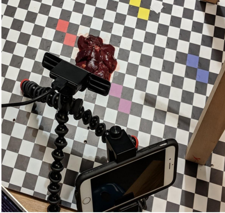
Figure 3.11: This is a photo of the setup used to scan some liver on the same calibration board that was used with the NextEngine scanner. As is clearly visible, the setup for this scanner is much simpler and requires much less manual effort than the NextEngine setup.
