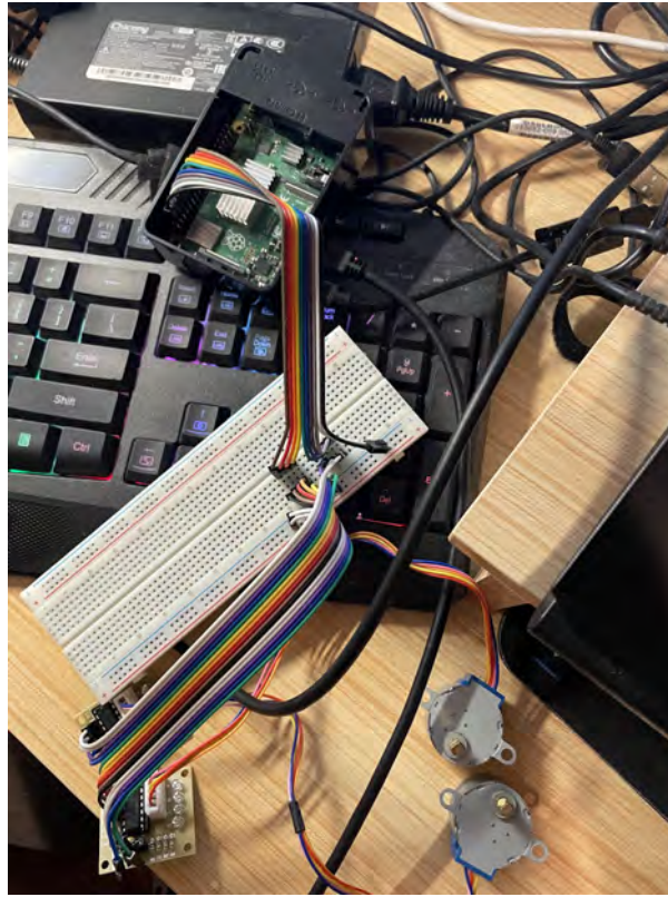
Fig. 5. Wiring of the motors
