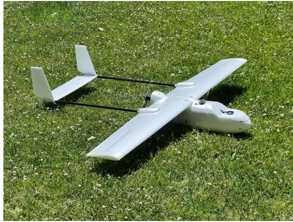
Fig. 3. Our built survey platform based on the Skyhunter 1800 fixed-wing airframe
