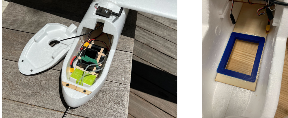
Fig. 4. Pictured Left: GoPro mounted in nose of fixed-wing, Right: Mounting hole for sensors
