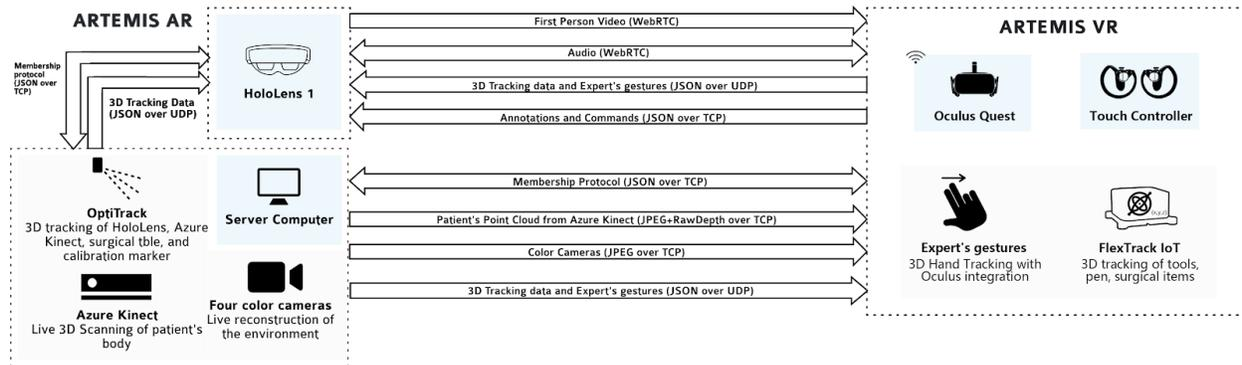
Figure 2. ARTEMIS is composed of two different environments: ARTEMIS AR and ARTEMIS VR . This diagram shows the origin and direction of data flowing and protocol usage from each environment
