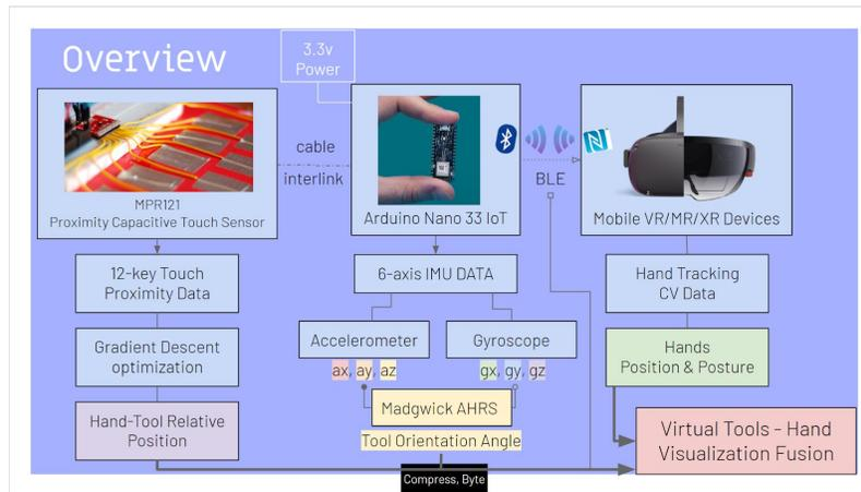
**Figure 6. FlexTrack Network overview. The FlexTrack IoT calculates only the orientation fusion algorithm and mostly serves as the data reporter of IMU data and touch key info, due to the limited computing power and battery life.**
