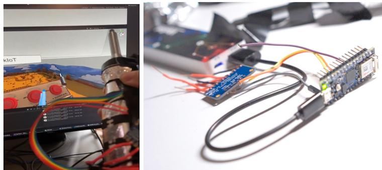
**Figure 5. ARTEMIS VR Input Interfaces - FlexTrack IoT. Expert surgeons interact with the interface through hands and a physical object attached with FlexTrack sensors. Left: a Tools integrated into FlexTrack API; Right: FlexTrack Sensor, connected with 4000mAh power bank**
