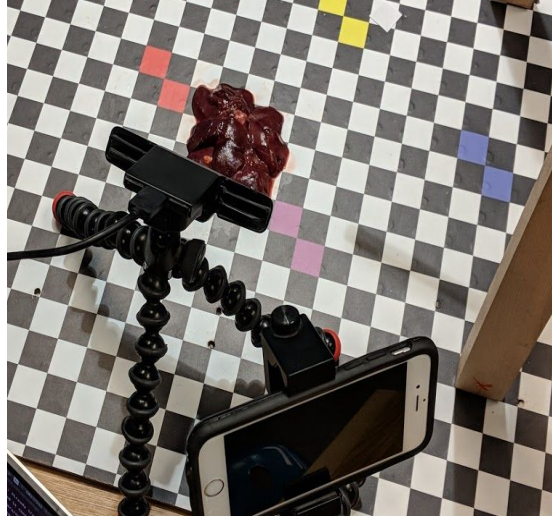
Figure 2.1 This is the setup that during the practice runs of data collection where we scanned a store-bought liver, as you can see in the image above the setup looks pretty simple and mobile, but the mount is not a perfect fit.
