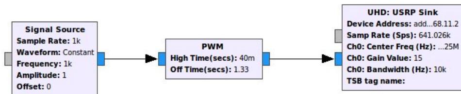
Figure 3-7. Transmitting Block Path from GNURadio Companion
