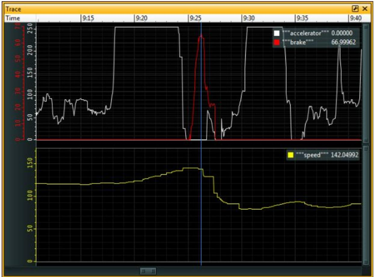
Fig. 4 Plot of accelerator position, brake position, and speed in a heavy braking zone
