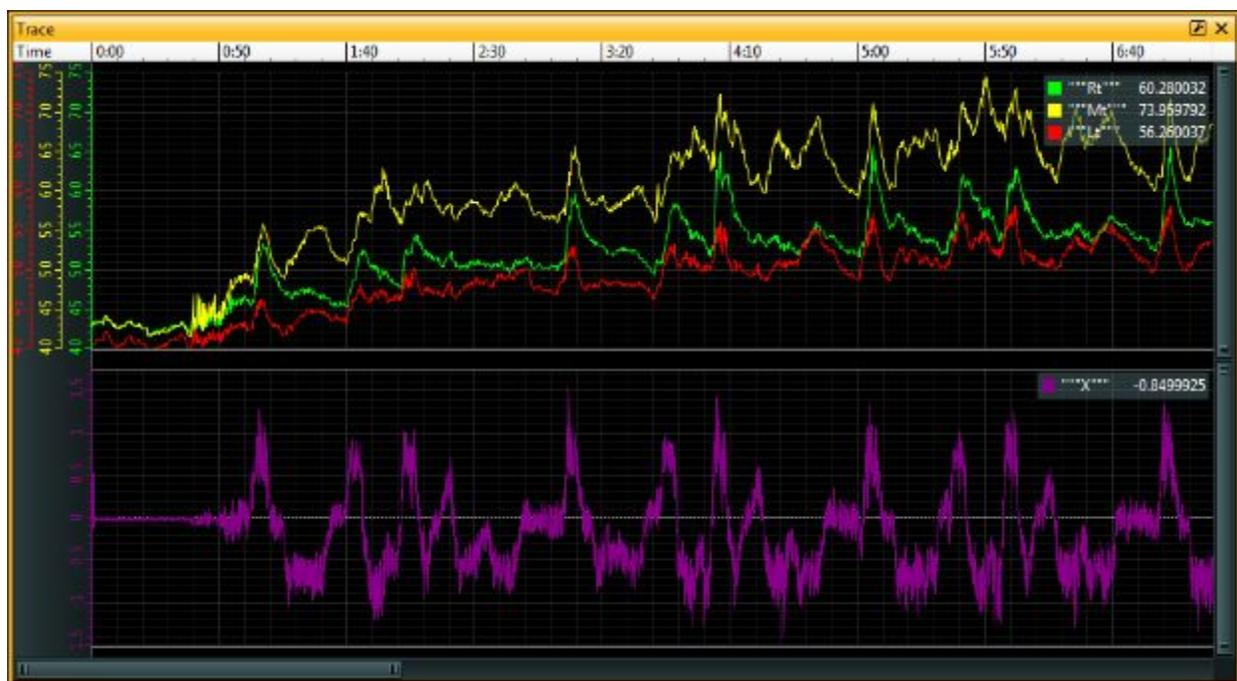
Fig. 5 Plots of tire temperature data (Rt, Mt, Lt) and lateral g-forces (X)
