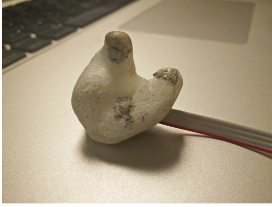
Fig. 5. The final iteration of the ear-EEG, which is made of rigid cast material from a mold impression.
