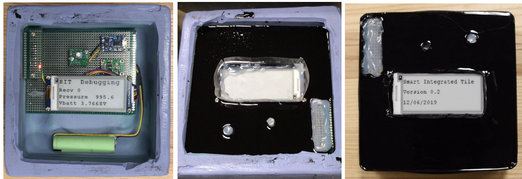
Figure 12: Potting process of the 2nd iteration
