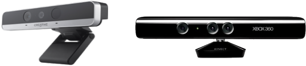
Fig.4 Comparison between Realsense(left) and Kinect(right) cameras.
