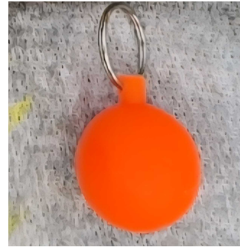
Fig. 2: Proof ball used as a fiducial marker by the Fishtechy mobile app.
