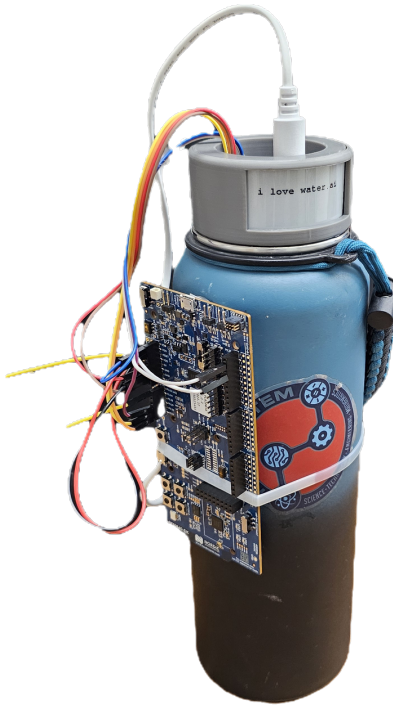
Fig. 7. Prototype with 3D-print of custom designed lid, TDS sensor, IMU, nrf52840dk and original non-flexible E-ink display
