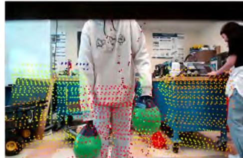
Fig. 5. Projected LiDAR points on image. Points colored from closest (red) to furthest (blue)
