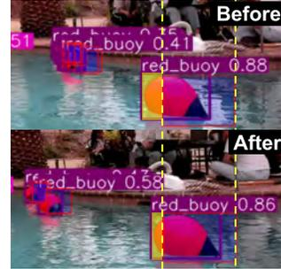
(b) Comparison in latency (offset labeled with yellow.) Optimized architecture (bottom) introduces lower latency than the initial choice (top).
