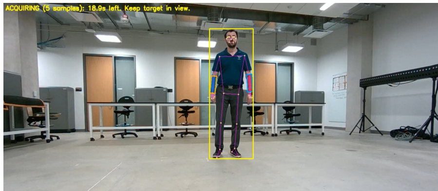
Fig. 7. Vision-based follower during the acquiring phase (indoor with good light conditions)
