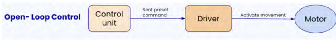
Fig. 8. Open Loop Control Diagram.
