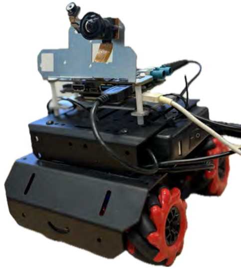
Fig. 3. The fully assembled robotic car, with the RB5 board mounted on the mBot Mega base.
