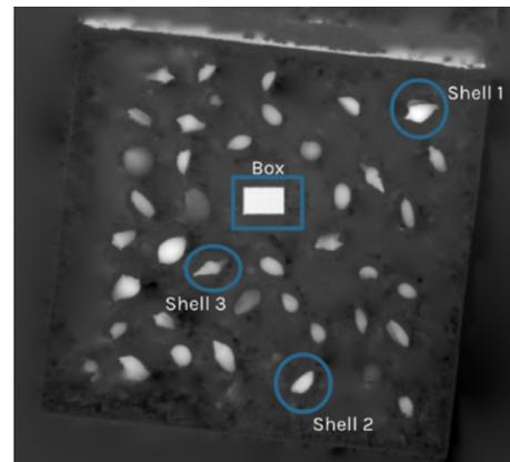
**Figure 4: Underwater testing board with box and shells of known dimensions.**
