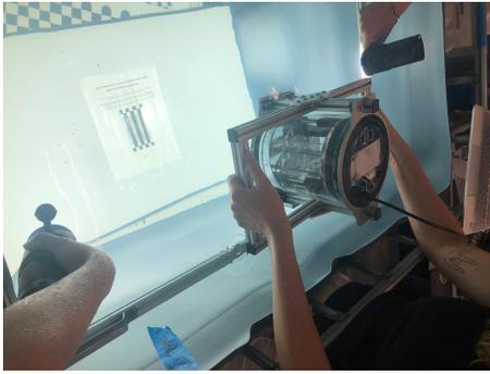
**Figure 2: Camera performing underwater targeted calibration over an open tank of freshwater**
