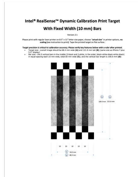
**Figure 1: Intel RealSense Dynamic Calibration target, used for targeted calibration**
