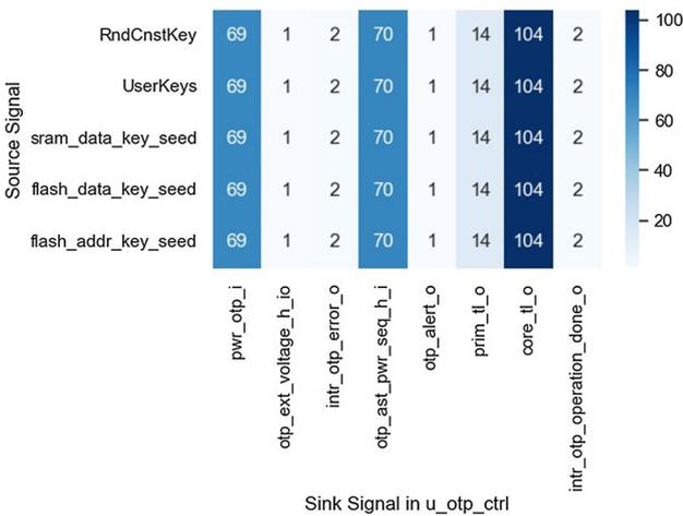
Fig. 6 Signal-to-signal conditional flow heatmap for an OpenTitan SoC module
