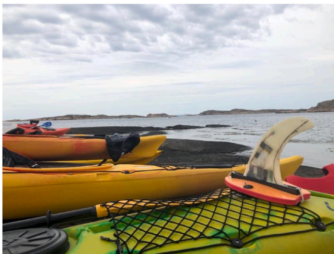
Fig. 6. Adaptation of the Smartfin for other watercraft (in this case, a sea kayak) by the fastening of a surf fin box to a small flotation device which is towed behind with a rope.
