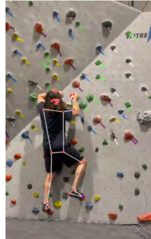
(b) MediaPipe landmark fault (inconsistency between hand landmark and hold)
