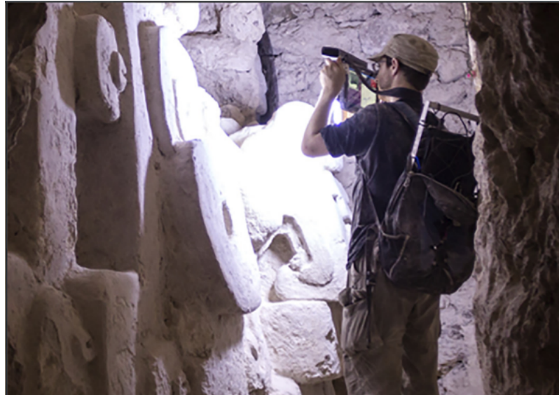
Fig. 1. The original scanning system with several cables leading into the user’s backpack in a cumbersome setup.
