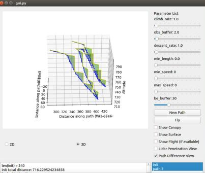
Here we have the original provably correct plot on the graph in blue, plotted against one of our smoothed paths in green. The green surface makes it easy to determine how exactly these two paths differ.
