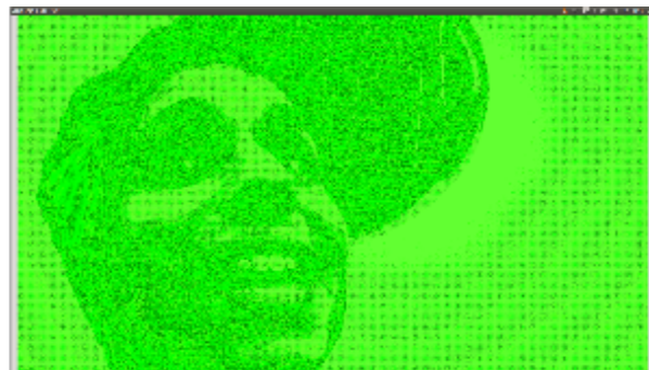
The raw image produced by the leopard imaging cameras was presented in a GR-bayer pattern. Needs to be decoded to RGB before computer vision algorithms can be applied.
