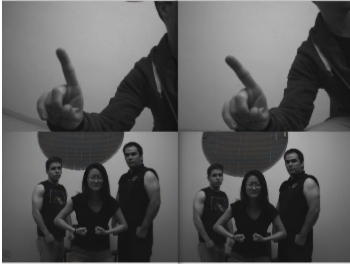
Top images: Time offset. The finger on the right is out of sync with the left and arrives later. The bottom images are properly synced.
