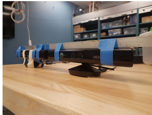
Figure 4.7: Setup for dual Kinect v2. This was a simple set up for testing purposes. RTAB-Map allows for the set-up to be more complex and can easily be changed. It does not require the intrinsic calibration that is needed for the
