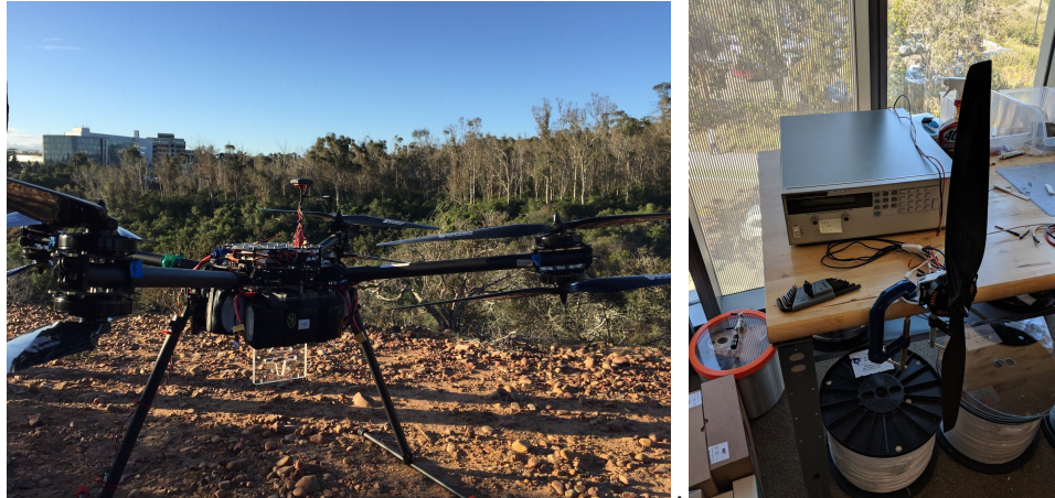
Figure 6. On the left is the assembled flight platform with batteries mounted underneath the centerpiece. On the right is an individual motor hooked up to the thrust test stand.
