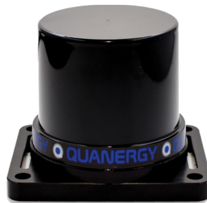
Figure 2. Quanergy M8 Lidar Sensor, our sensor of choice.
